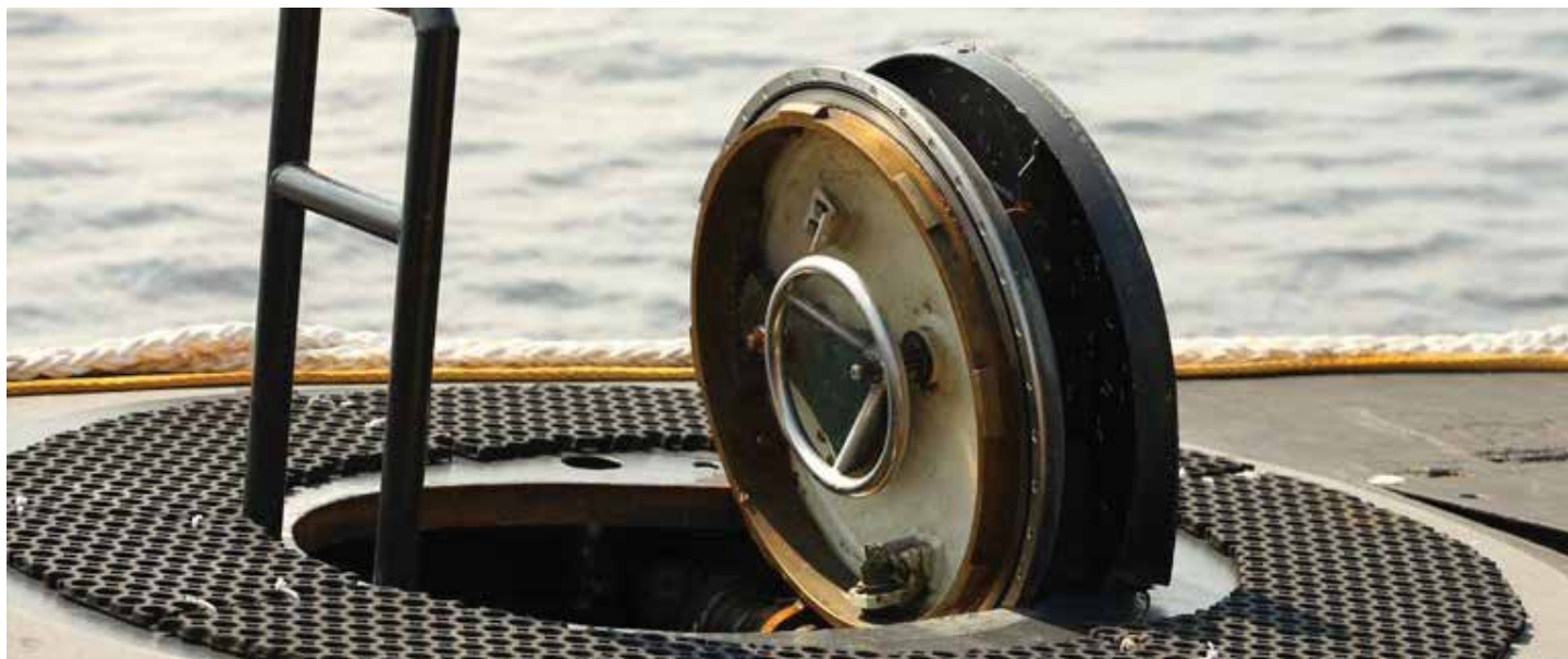
Figure 1: An Actuated Part Subjected to Extreme Seawater Environments, Requiring High-Performance Lubricants That Are Also Sailor-Safe (Source: © mrivserg-stock.adobe.com).
