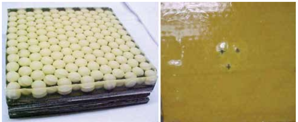
Figure 3: Ceramic Spheres Embedded in Elastomer (Left); Front-Side After Penetration by Three 0.50-cal. AP Rounds Falling Within 2-inch Circle (Stanag 4241 Bullet Impact Test), Showing Small Holes in Kevlar Top Layer (Right). The Damage Zone Is Less Than the Bullet Diameter Because the Elastomer Contains the Ceramic Granulated by the Projectile (Source: NRL).
