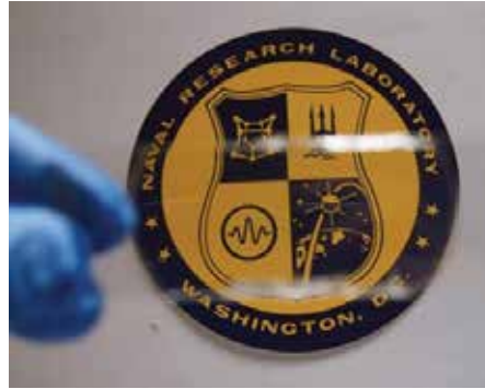
Figure 6: Transparent Elastomer Used for Coating (Source: NRL).
