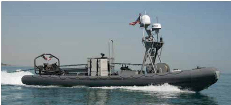
Figure 1: Remotely Piloted USV in a Mine Hunting Exercise (Source: U.S. Navy Photo by Ken Rose).
