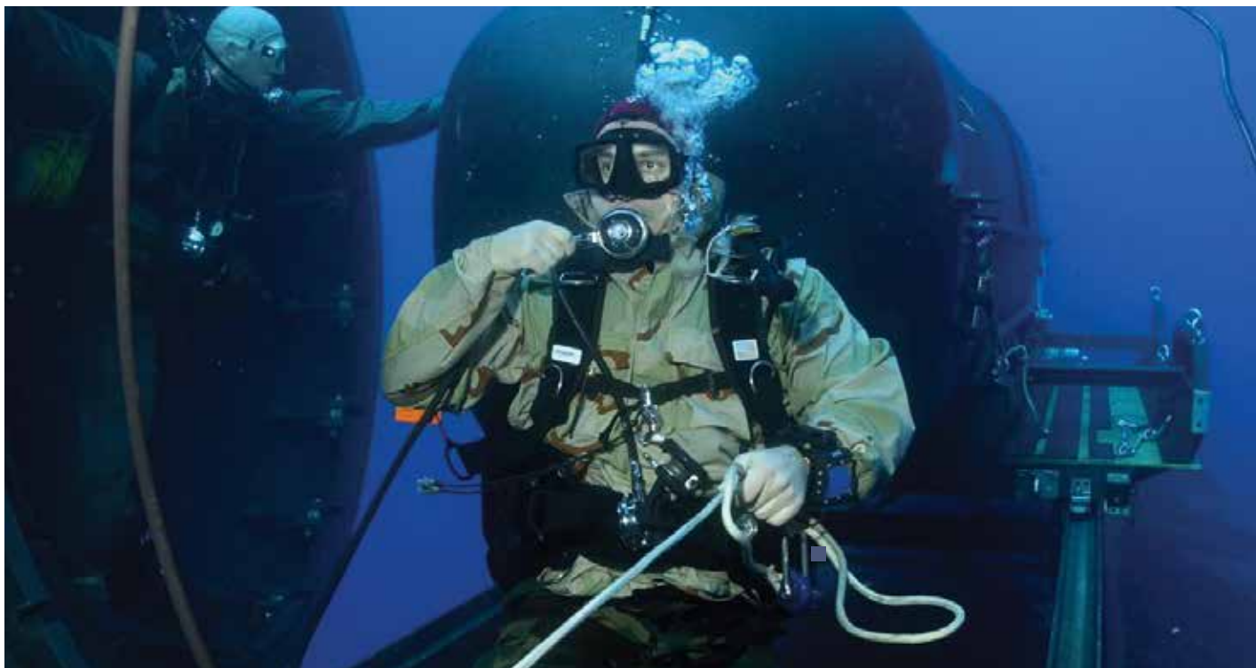
Figure 2: Navy SEAL in a Dry Deck Shelter on the Back of a Los Angeles-Class Submarine. Lubrication of Actuated Parts in the Shelter Is Critical to Personnel Safety (Source: U.S. Navy Photo, Chief Photographer's Mate Andrew Mckaskle).
