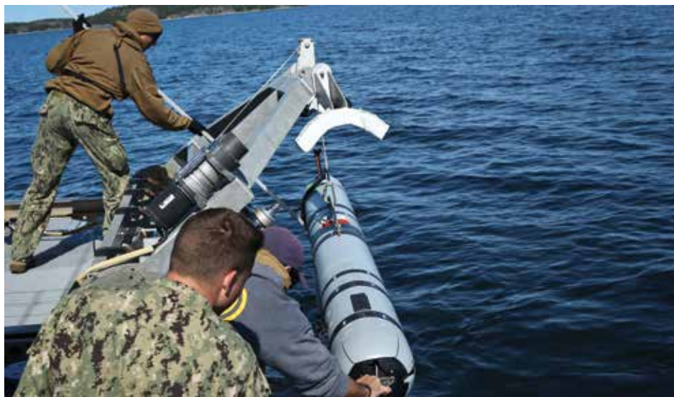
Figure 2: UUV Being Prepared to Search for Mines During Exercise (Source: U.S. Navy Photo by Mass Communication Specialist 1st Class A. Henry).
